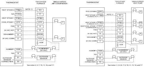
Modulating and 2-Stage Furnace with Single-Speed Air Conditioner
