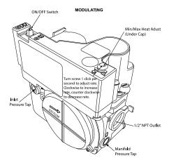
Fig. 63 - Gas Valve without Tower Pressure Ports
