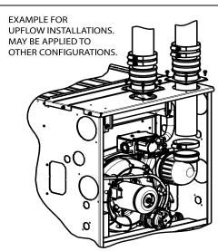
Fig. 50 – Sample Inlet Air Pipe Connection for Polypropylene Venting Systems
