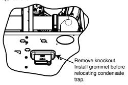
Fig. 17 – Horizontal Drain Trap Grommet
