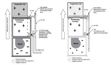
Fig. 11 – Example of Field Drain Attachment
