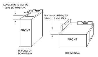
Fig. 18 - Furnace Pitch Requirements
