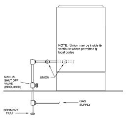
Fig. 31 – Typical Gas Pipe Arrangement
