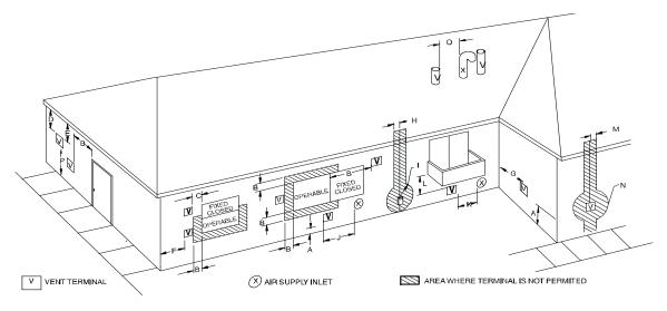
Fig. 44 – Direct Vent Termination Clearance
