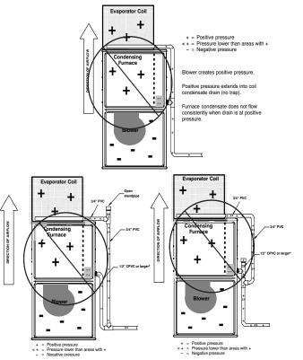
$\textbf{Fig. 12-Example of Field Drain Attachment (Not Allowed)}^{\text{A14532}}$
