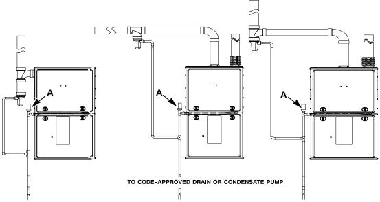
Recommend "T" fitting with 4-inch minimum height standpipe (A) of same diameter or larger extending upward.
