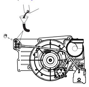
Fig. 60 – Priming Condensate Trap (Appearance May Vary)
