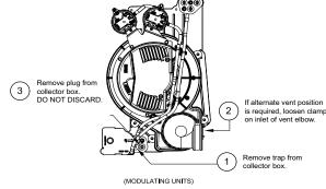
Unconverted Factory Trap Configuration
