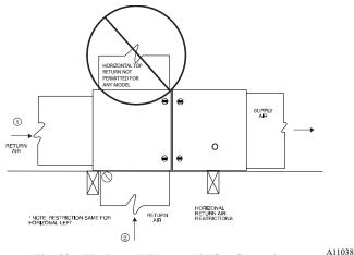
Fig. 22 – Horizontal Return Air Configurations and Restrictions
