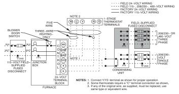
Fig. 32 – Typical Field Wiring Diagram
