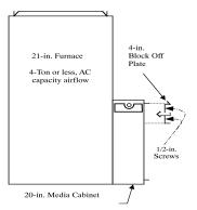
Media Cabinet Installation Option for 4-Ton or Less A/C Capacity
