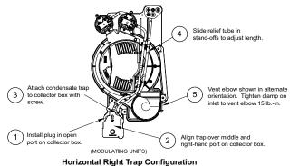
Fig. 10 – Horizontal Right Trap Configuration (Appearance May Vary) A11278B
