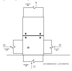
Fig. 20 – Upflow Return Air Configurations and Restrictions  $^{\rm A11036}$
