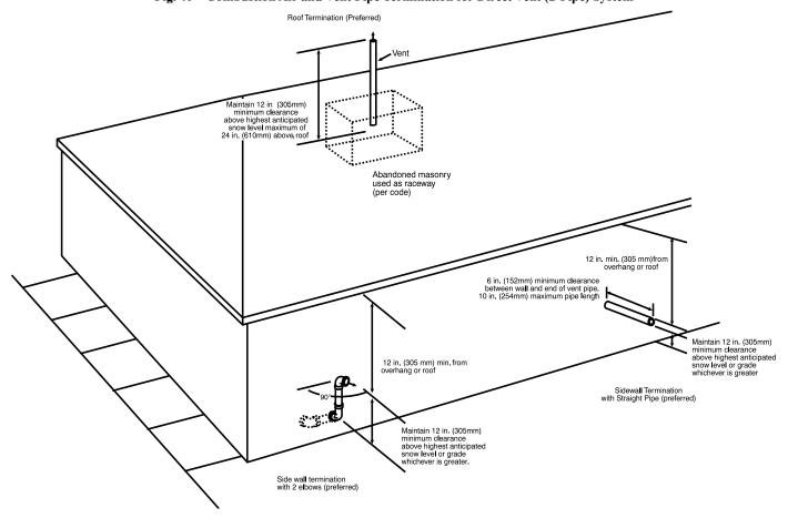
Fig. 41 – Vent Pipe Termination for Non-Direct Vent and Ventilated Combustion Air System
