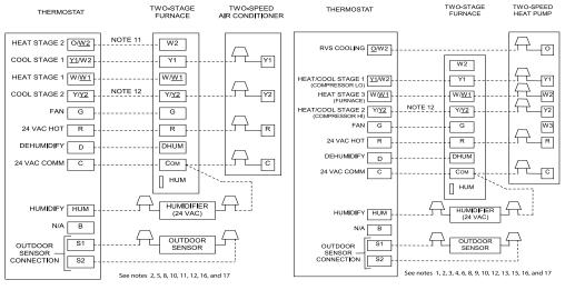
Modulating and 2-Stage Furnace with Two-Speed Air Conditioner Modulatin
