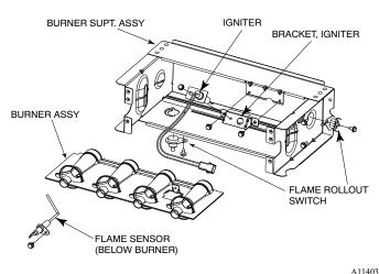
Fig. 66 - Burner Assembly
