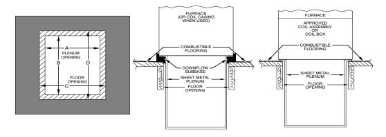
Fig. 24 - Installation on Combustible Flooring
