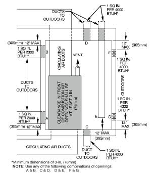
L12F012 Fig. 6 – Air for Combustion, Ventilation, and Dilution for Outdoors
