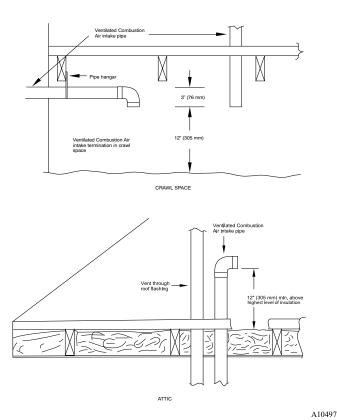
Fig. 47 – Vent Terminations for Ventilated Combustion Air Size the Vent and Combustion Air Pipes
