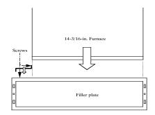
14-3/16-in. Furnace with Filler Plates, Off-Set to Right
