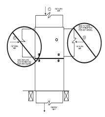
Fig. 21 – Downflow Return Air Configurations and Restrictions
