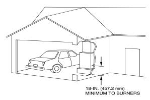
Fig. 5 – Installation in a Garage
