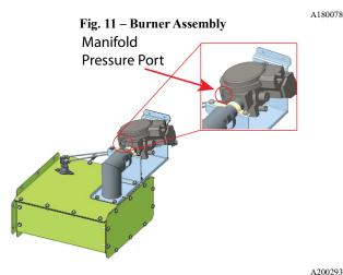
Fig. 12 – BurnerBox/Gas Manifold Assembly
