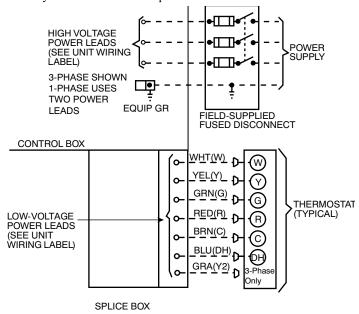
Fig. 10 - High- and Control-Voltage Connections
