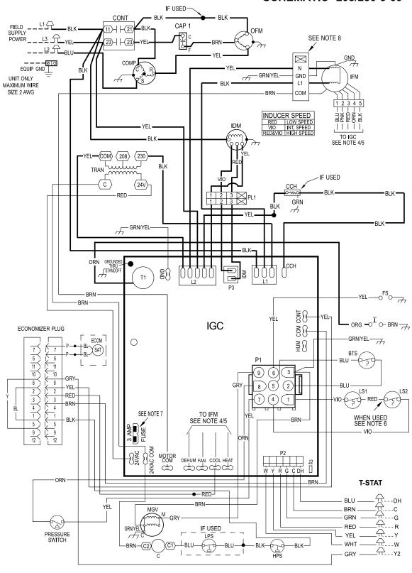
Fig. 17 – 208/230-3-60 Ultra Low NOx Connection Wiring Diagram
