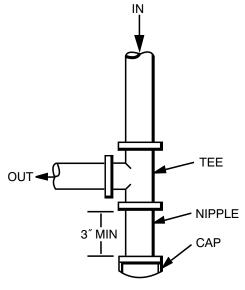
Fig. 8 – Sediment Trap
