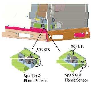
Fig. 20 – Burner Thermal Switch (BTS) (Ultra Low NOx)
