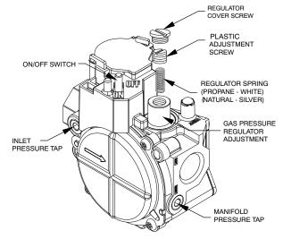
Fig. 13 – Standard Single-Stage Gas Valve
