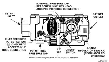
Fig. 14 – Single-Stage Gas Valve with Tower Pressure Ports
