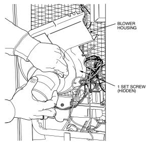
Fig. 23 - Removal of Motor and Blower Wheel
