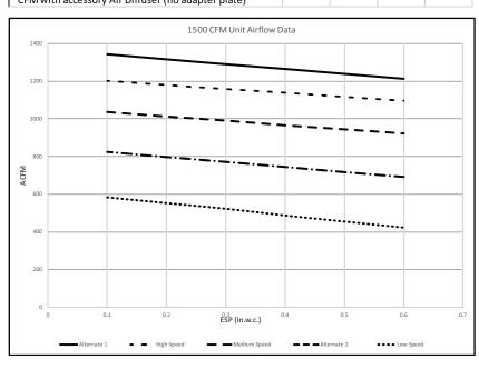
Fig. 5 – Static Pressure - 015 Size
