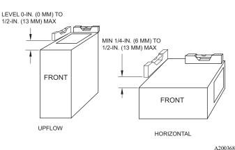
Fig. 31 – Furnace Pitch Requirements
