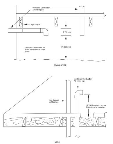
Fig. 63 – Vent Terminations for Ventilated Combustion Air
