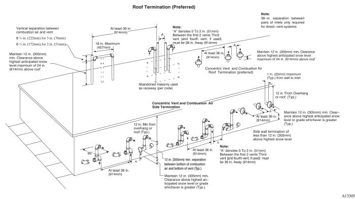
Fig. 61 - Combustion Air and Vent Pipe Termination for Direct Vent (2-Pipe) System
