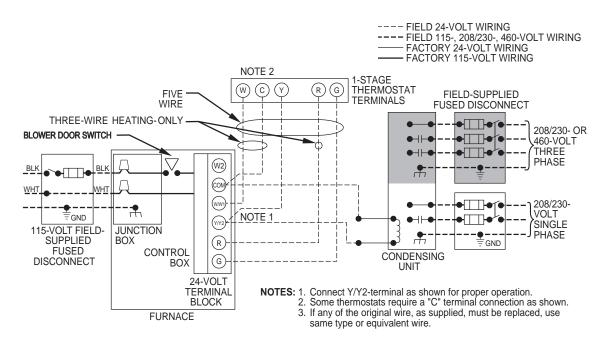
Fig. 41 – Typical Single-Stage Wiring Diagram
