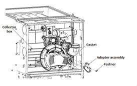
Fig. 14 – Upflow Example of Trap Adapter Installation
