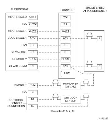
Fig. 43 – 1-Speed Variable Furnace with Single-Speed Air Conditioner
