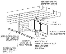
NOTE: FURNACE SHOWN IS A DIRECT VENT APPLICATION. REFER TO THE VENTING SECTION FOR ALLOWABLE VENT CONFIGURATIONS. NOTE: (N COIL ONLY, ADD 8" SEPARATION BETWEEN COIL & FURNACE FOR ALL OTHER UNSHIELDED COILS) SEE EVAPORATOR COIL SPACER OR SHIELD REQUIREMENTS.
