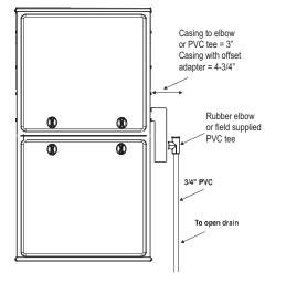
Fig. 7 – Trap Clearance in Upflow Application
