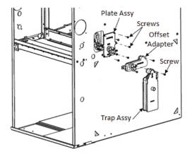
Fig. 16 – Upflow - Offset of Condensate Drain
