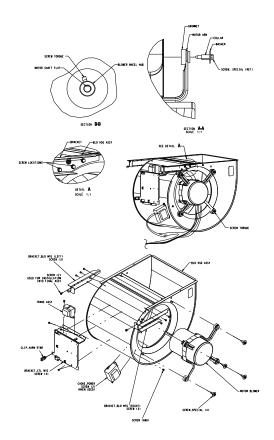
Fig. 70 - Blower Assembly on 100C21--22
