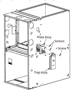
Fig. 15 – Upflow Condensate Drain
