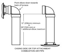
COMBUSTION AIR PIPE (NON-DIRECT VENT FOR ALL MODELS EXCEPT MODULATING UNLESS INSTALLED IN ATTIC OR CRAWL SPACE)
