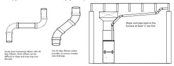
Fig. 52 – Near Furnace Vent Connections
