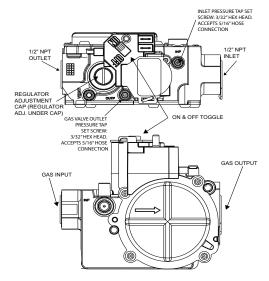
Fig. 67 – Gas Control Valve
