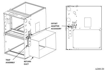
Fig. 18 – Upflow Right Side Return Configuration - Required Upflow Offset Installation
