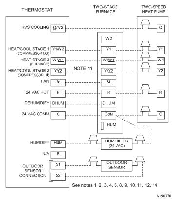
Fig. 46 – 1-Speed Variable Furnace with Two-Speed Heat Pump (Dual Fuel)
