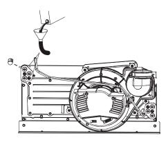
Fig. 65 – Prime Condensate Trap
