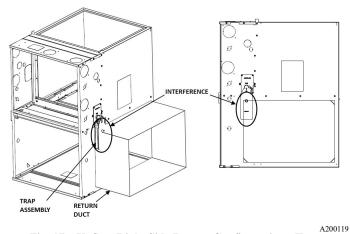
Fig. 17 – Upflow Right Side Return Configuration - Trap Interference
