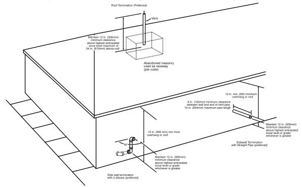
Fig. 62 - Vent Pipe Termination for Non-Direct Vent and Ventilated Combustion Air System
