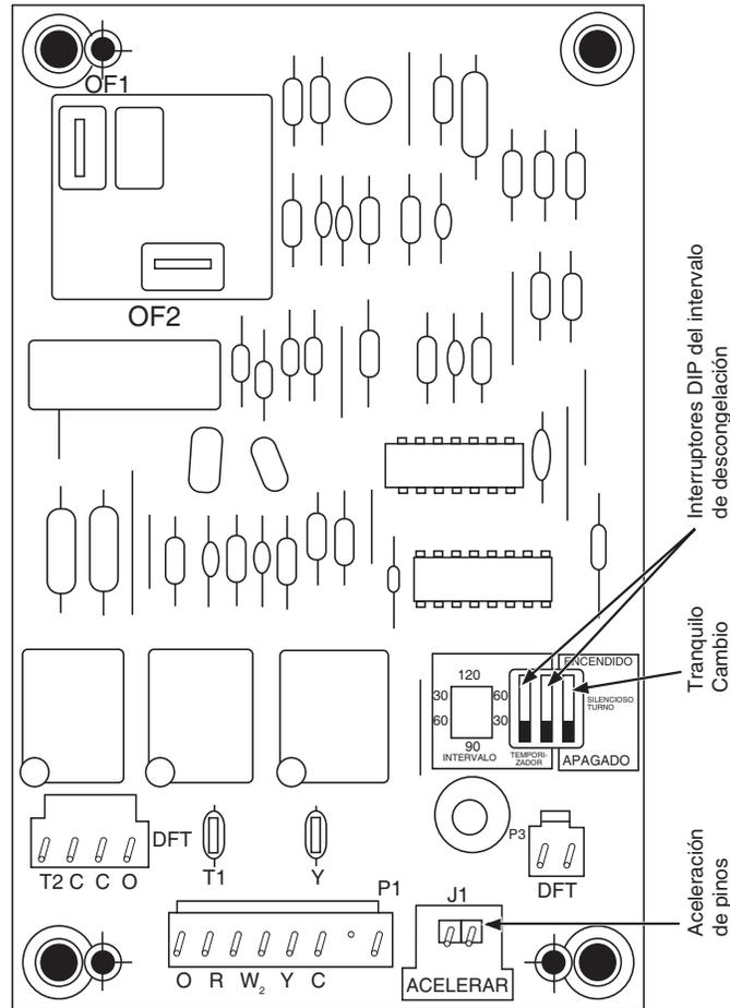
Fig. 11 – Placa de control Quiet Shift-2
