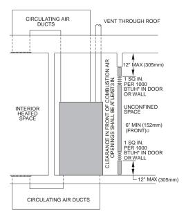
\*Minimum opening size is 100 in.2 with minimum dimensions of  $3^{A03175}$  (76 mm).
