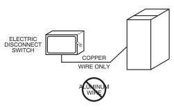
Fig. 25 – Field-Supplied External Electrical Box on Furnace Casing J-BOX RELOCATION
