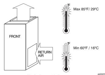
Fig. 3 – Return Air Temperature
