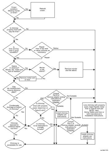
Fig. 30 – Chimney Inspection Chart
