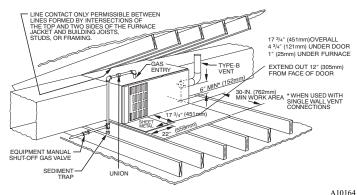
Fig. 14 – Typical Attic Installation
