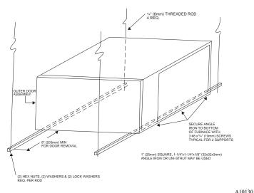
Fig. 15 – Horizontal Unit Suspension
