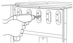
Fig. 50 – Cleaning Heat Exchanger Cell
