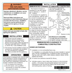
Fig. 2 – Clearances to Combustibles
