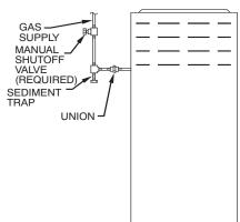
Fig. 23 - Typical Gas Pipe Arrangement
