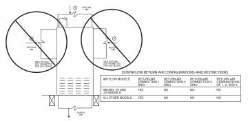
Fig. 18 – Downflow Return Air Configurations and Restrictions  $^{A02163}\,$
