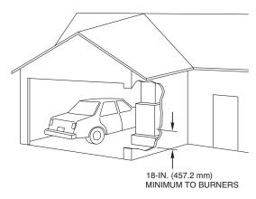
Fig. 5 – Installation in a Garage
