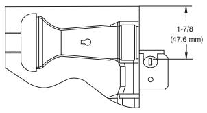
Fig. 48 – Igniter Position-Top View
