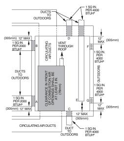
\*Minimum dimensions of 3 in. (76 mm).
