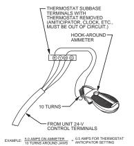
Fig. 47 – Amp. Draw Check with Ammeter Table 13 – Gas Rate (Cu Ft./Hr.)
