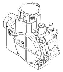
Fig. 21 – Gas Control Valve
