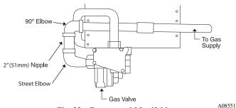
Fig. 22 – Burner and Manifold
