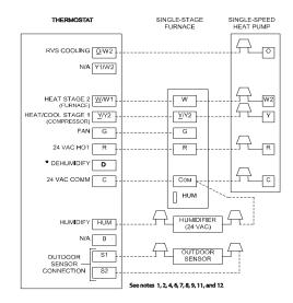
Single-Stage Furnace with Single-Speed Air Conditioner
