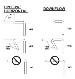
Fig. 17 – Duct Flanges
