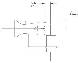
Fig. 49 – Igniter Position-Side View
