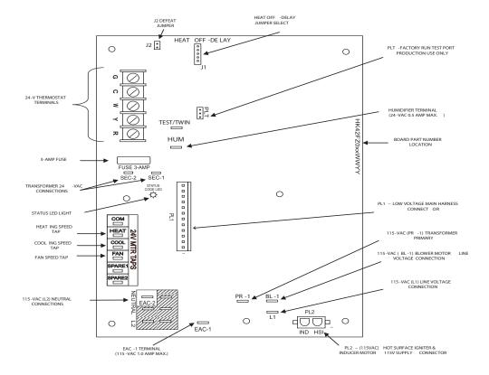
Fig. 28 - Furnace Control
