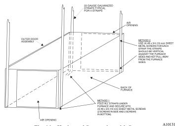
Fig. 16 - Horizontal Suspension with Straps
