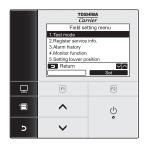
Push the [ ∧ ∧] / [ ∨ ∨] button to select "DN setting" on the "Field setting menu" screen, then push the "Set" Set" [ P F2] button.
