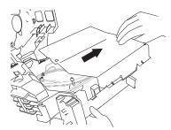
4 Remove the electrical control box cover and set bit1 of SW01 on the board to ON. (Do not touch SW02 as it is used for other setting.)
