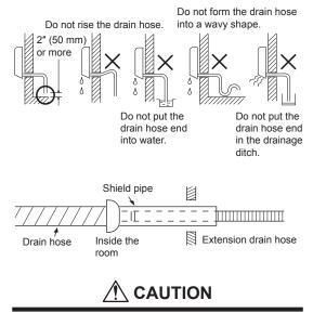
Arrange the drain pipe for proper drainage from the unit.
