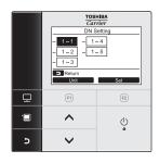
2 The indoor UNIT No. in the group control is displayed in order. Select the indoor unit of which setup is changed. In this time, the position of the indoor unit of
