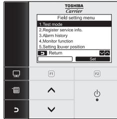
Push the [^] / [v] button to select “DN setting” on the “Field setting menu” screen, then push the “Set” [F2] button.
