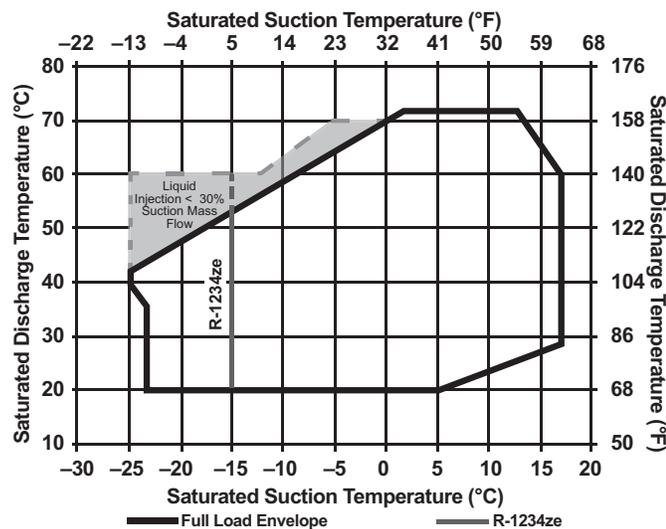
**Fig. 5 — Full Load Operating Envelope with Liquid Injection**
