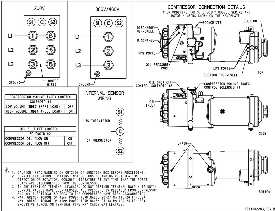
**Fig. 13 — Compressor Connection Details**
