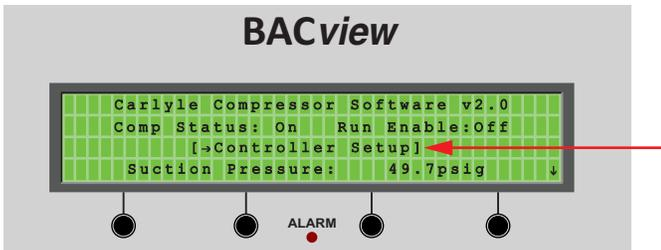
**Fig. 11 — Controller Setup Menu**
