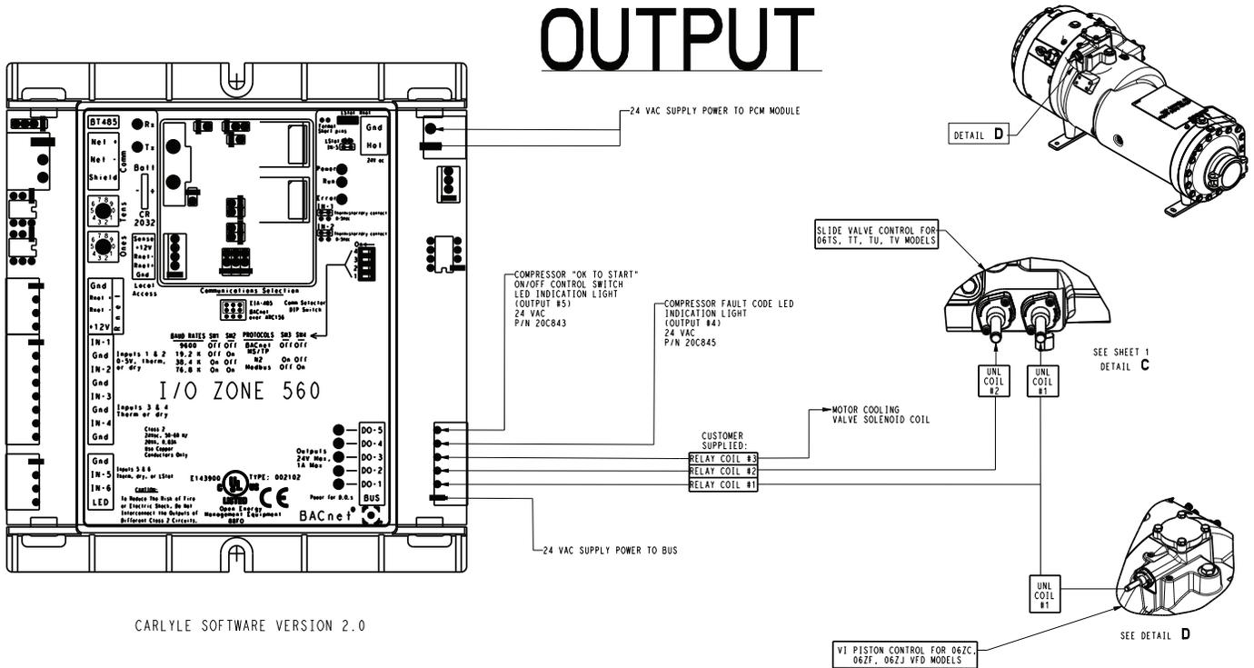
Fig. 9 — PCM Inputs and Outputs
