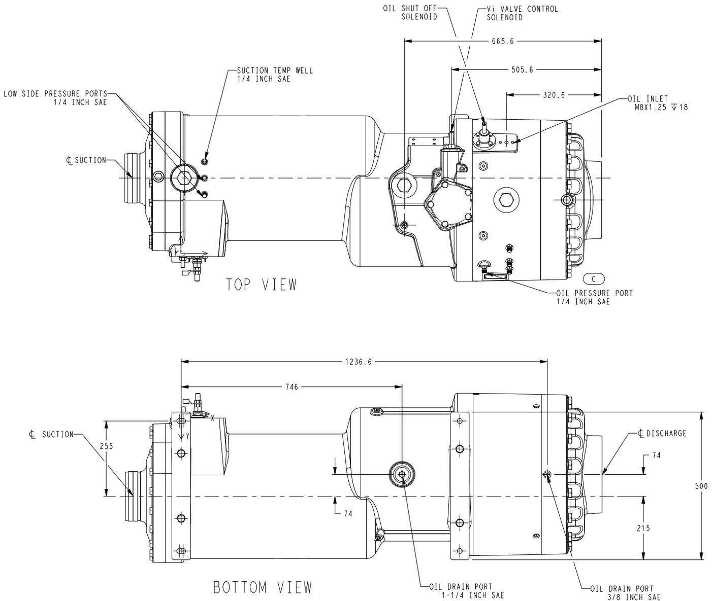
Fig. 4 — Compressor Physical Data and Connections (06ZJ, Frame 3) (cont)
