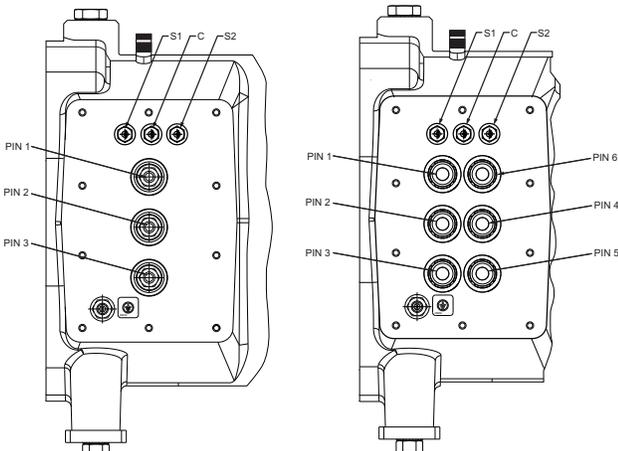
**Fig. 16 — Motor Lead Connections**
