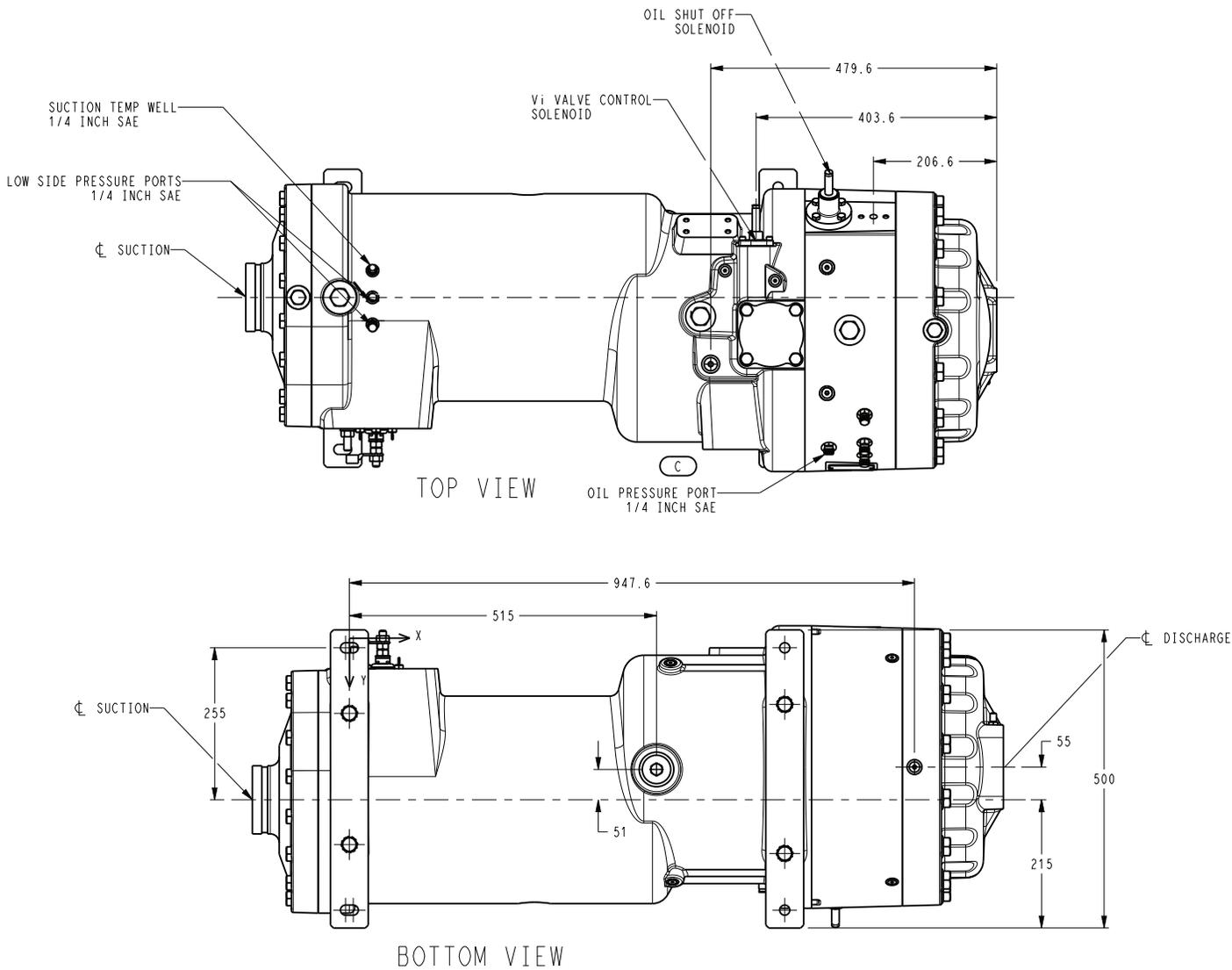
**Fig. 2 — Compressor Physical Data and Connections (06ZC, Frame 1) (cont)**
