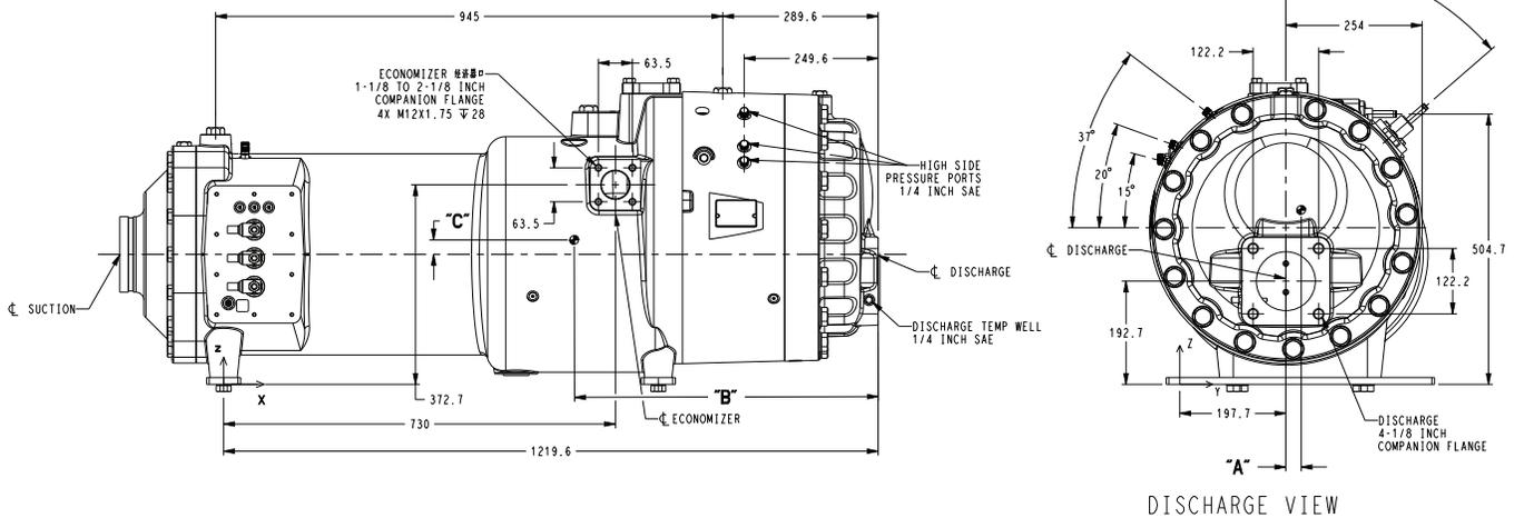
Fig. 3 — Compressor Physical Data and Connections (06ZF, Frame 2)
