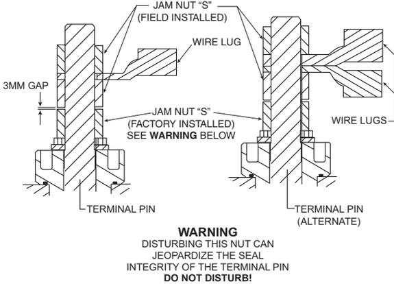
**Fig. 15 — Terminal Pin Cross-Section**
