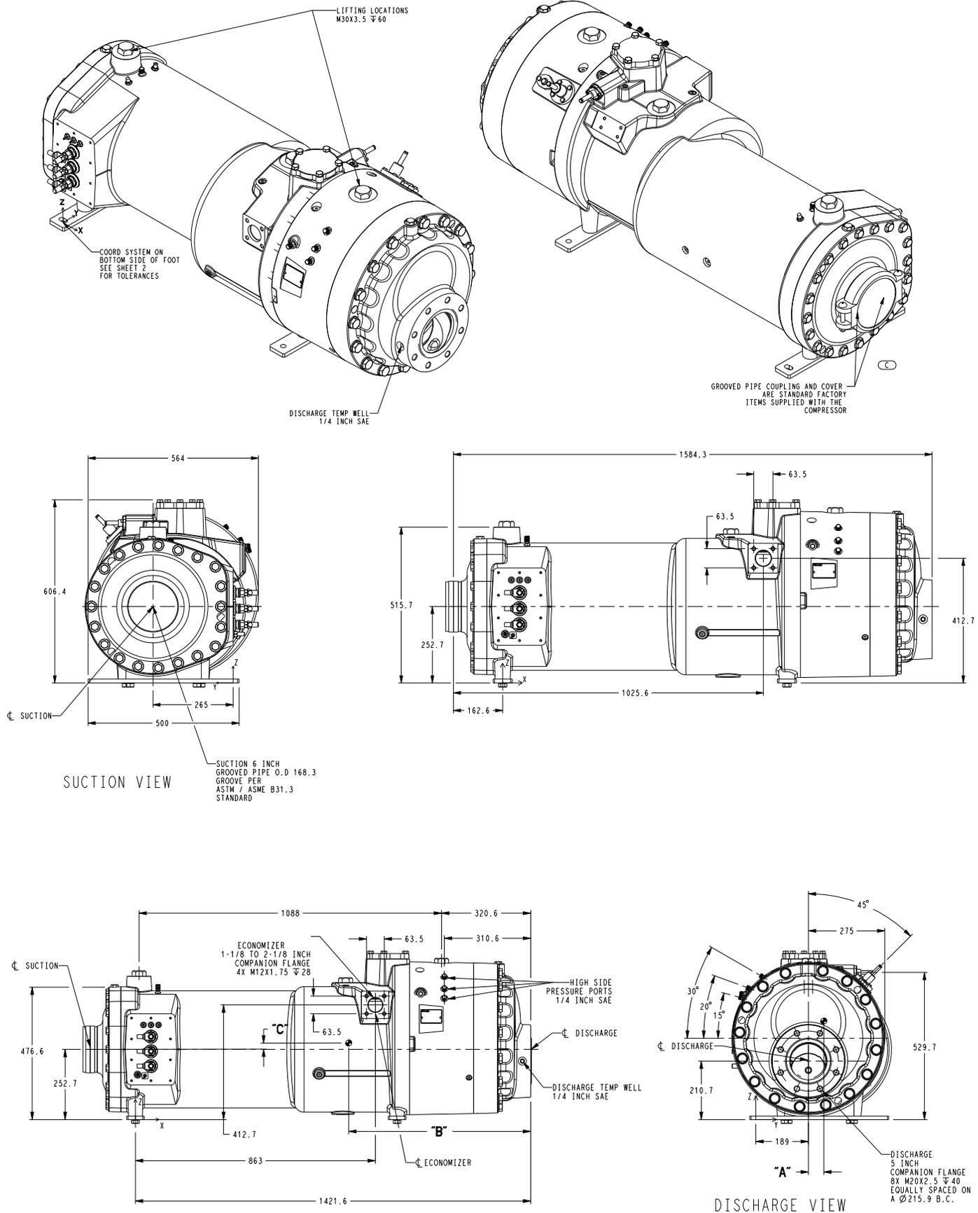
Fig. 4 — Compressor Physical Data and Connections (06ZJ, Frame 3)
