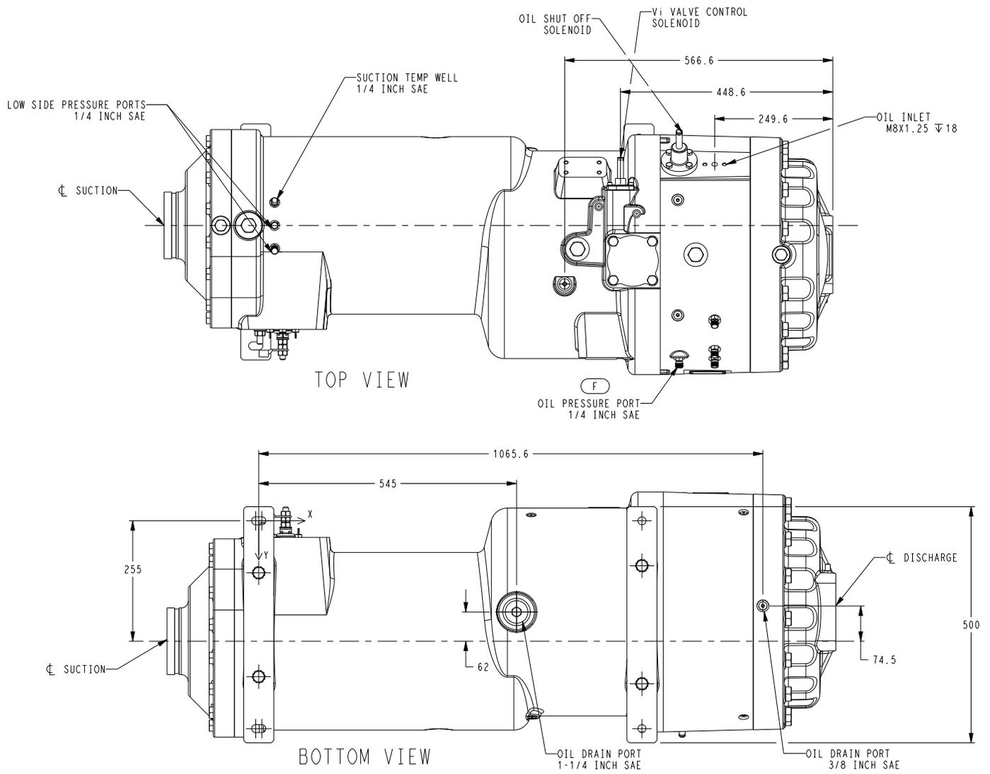
**Fig. 3 — Compressor Physical Data and Connections (06ZF, Frame 2) (cont)**
