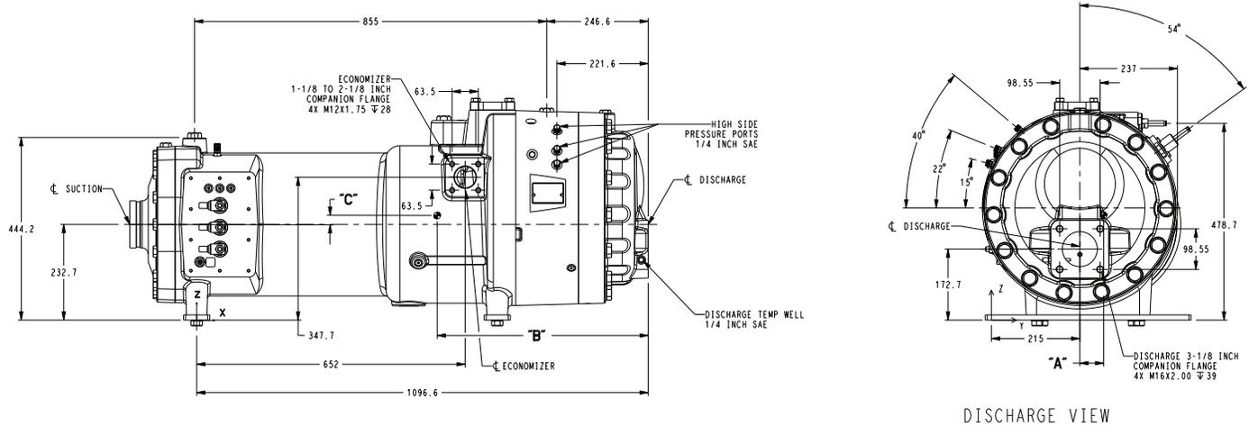
**Fig. 2 — Compressor Physical Data and Connections (06ZC, Frame 1)**
