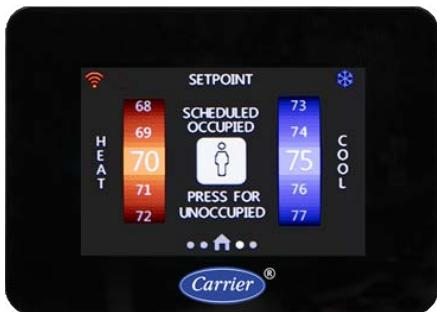
Use this screen to view, adjust, or hold heat and cool setpoints. Use the wheels to adjust setpoints. Drag a wheel up or down or tap the top or bottom of the wheel to increase or decrease by 1 increment.
