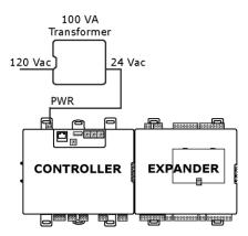
• Wired to the I/O Bus port for communication and then wired to an external transformer for power
