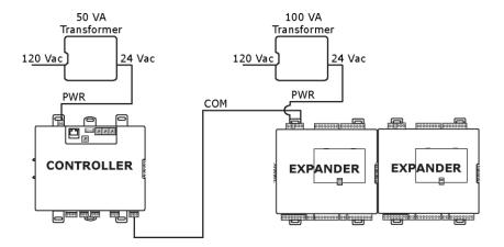
The following configuration shows a combination of connections using the I/O bus edge connector and daisy-chained wiring to the I/O Bus ports.
