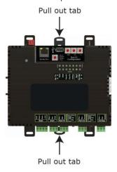
2 Place the controller on the DIN rail so that the rail is in the trough on the back of the controller.
