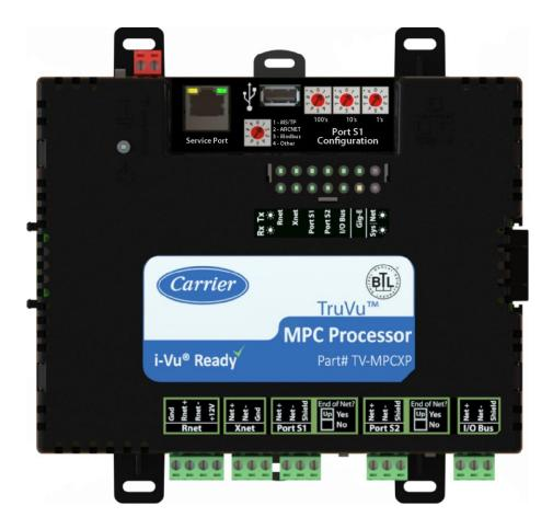
The TV-MPCXP has 4 physical ports for BACnet or Modbus communication:
