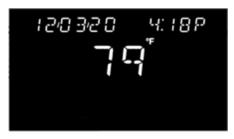
The banner scrolls through date and time, humidity, outdoor air temperature, if configured, and any active faults or system events. The room temperature is prominently displayed.
