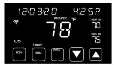
The center portion of the screen displays the current space temperature in whole degrees. The default temperature scale is °F, but can be changed to °C in the *Installer settings* (page 30).
