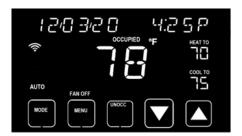
When changing the setpoints in **AUTO** mode, the setpoint modified by the up and down arrows is the last setpoint that was changed. To adjust the opposite mode setpoint, touch the setpoint value on the display. **HEAT TO** or **COOL TO** flashes above the setpoint and can be changed by using the up and down arrows. The setpoints enforce a 2-degree deadband. Setpoints in °F are displayed in whole degrees. Setpoints in °C are displayed with half degree resolution.
