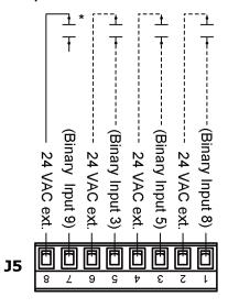
The terminals for Inputs 3, 5, and 8 are available for use in place of the flying wire leads at Molex connectors J1 and J2 identified below:
