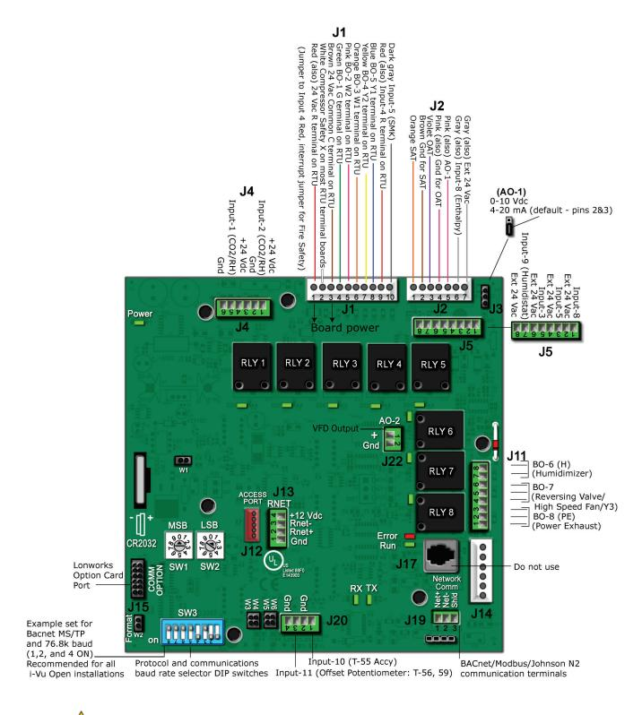
**CAUTION** If there is a jumper on the Format pins and power is cycled to the controller, all Modbus, N2, and LonWorks points will be lost.
