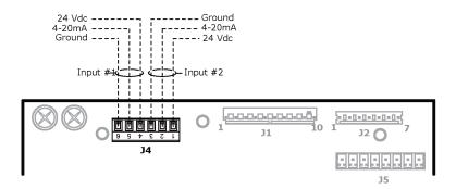
**NOTE J4** Analog Inputs 1 and 2 may be set for the following device types:
