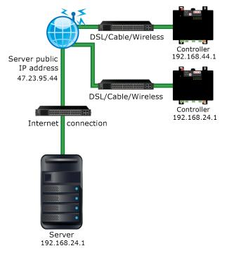
In this example, each controller needs to communicate with only the i-Vu® Pro server so their BACnet firewall's whitelist should have only the server's public IP address. The controllers do not need to communicate with each other.
