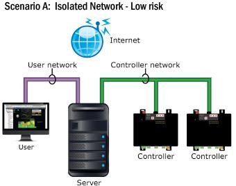
Do not permanently expose the i-Vu® Pro server or the BACnet network to the Internet. You can, however, allow users to access the i-Vu® Pro server through a secure VPN connection. If a NAT router or firewall is present on the LAN for other purposes, it should not have any ports forwarded to the i-Vu® Pro server or any controllers.
