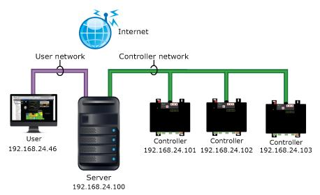
In this example, each controller's BACnet firewall should allow BACnet communication from the i-Vu® Pro server's IP address and the controller's IP addresses. The user at 192.168.24.46 should not be allowed BACnet communication with the controllers.
