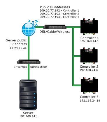
In this example, the controllers need to communicate with the i-Vu® Pro server and each other. The controllers are the only devices on the site's private network, or other devices present are benign.
