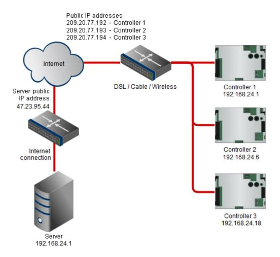
In this example, the controllers need to communicate with the i-Vu® Pro server and each other. The controllers are the only devices on the site's private network, or other devices present are benign.
