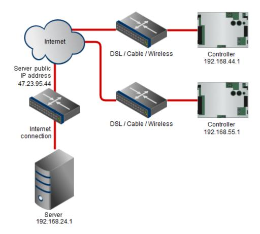
In this example, each controller needs to communicate with only the i-Vu® Pro server so their BACnet firewall's whitelist should have only the server's public IP address. The controllers do not need to communicate with each other.
