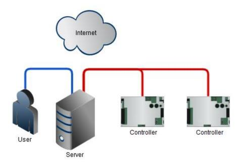
Do not permanently expose the i-Vu Pro server or the BACnet network to the Internet. You can, however, allow users to access the i-Vu Pro server through a secure VPN connection. If a NAT router or firewall is present on the LAN for other purposes, it should not have any ports forwarded to the i-Vu Pro server or any controllers.
