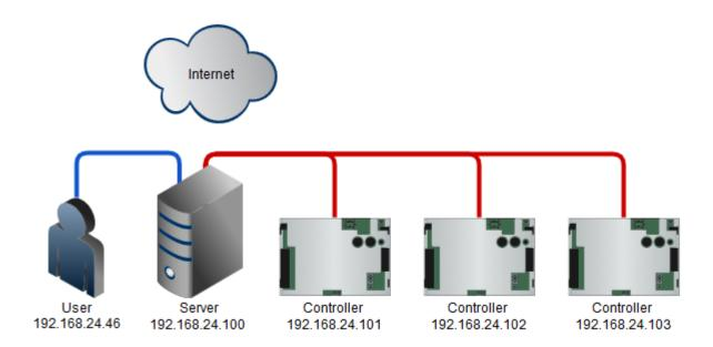
In this example, each controller's BACnet firewall should allow BACnet communication from the i-Vu® Pro server's IP address and the controller's IP addresses. The user at 192.168.24.46 should not be allowed BACnet communication with the controllers.
