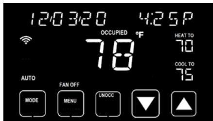
When changing the setpoints in **AUTO** mode, the setpoint modified by the up and down arrows is the last setpoint that was changed. To adjust the opposite mode setpoint, touch the setpoint value on the display. **HEAT TO** or **COOL TO** flashes above the setpoint and can be changed by using the up and down arrows. The setpoints enforce a 2-degree deadband. Setpoints in °F are displayed in whole degrees. Setpoints in °C are displayed with half degree resolution.
