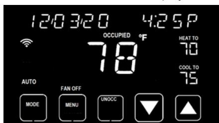
You can change the fan setting by pressing **MENU** and then the current fan setting is displays.
