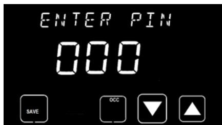
This screen has an **OCC/UNOCC** button to temporarily override the program schedule settings without knowing the PIN. The PIN must be entered for all other thermostat changes. Pressing the **OCC/UNOCC** button temporarily overrides the program schedule settings with the occupied or unoccupied settings. This override remains active until the next time range in the program schedule or until the **MAX HOLD** time expires.
