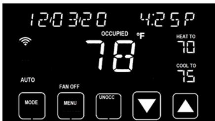
The center portion of the screen displays the current space temperature in whole degrees. The default temperature scale is °F, but can be changed to °C in the *Installer settings* (page 24).
