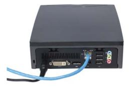
If you are using the USB Adapter (CCN or Open) to connect to your network, plug the adapter into the USB port and connect to your network. You can only use one adapter on the web server.
