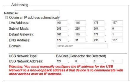
In cases where the DHCP Server will not assign 2 IP addresses and the i-Vu® system uses both a USB Adapter and external routers, DHCP will not work. You must configure the i-Vu® system with static IP addresses. See Configure the i-Vu® system using a static IP address.
