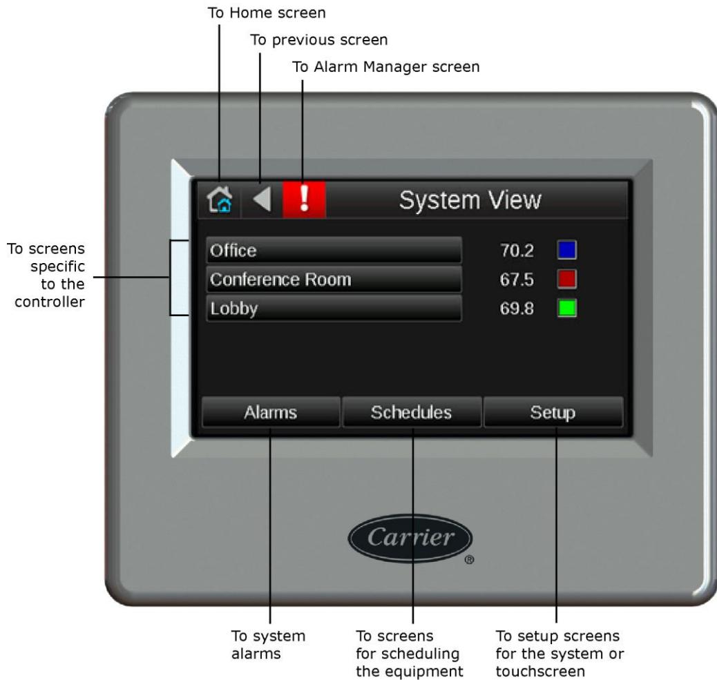
The System Touch has built-in temperature and humidity sensors. You can use their values to control equipment. You can also wire an external thermistor to the System Touch and use its value instead of the built-in temperature sensor's value.
