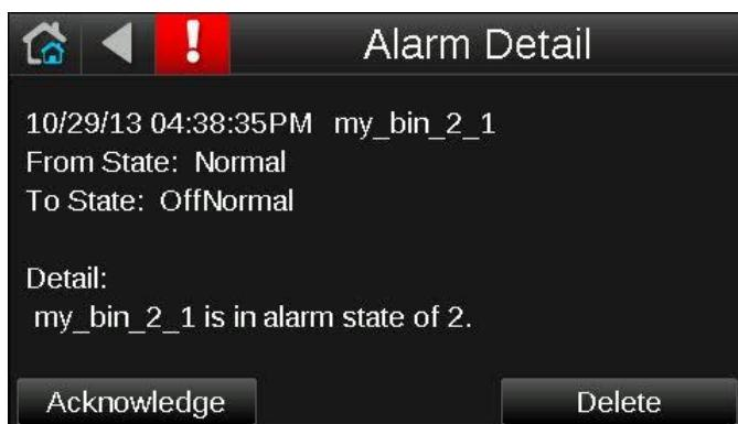
**NOTE** The System Touch can hold up to 100 alarms. When the System Touch reaches 100, the oldest alarm is deleted when a new alarm comes in.
