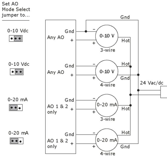
6 Set the **AO Mode Select** jumper to the type of device you are wiring the output to.
