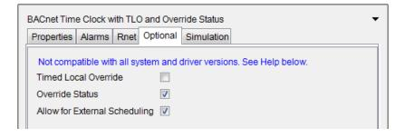
The **ext** input tells the Schedule Microblock to use the external "commanded to" input instead of the internal schedule. When the top BV is on, the **cmd** input determines the schedule status. See example below.
