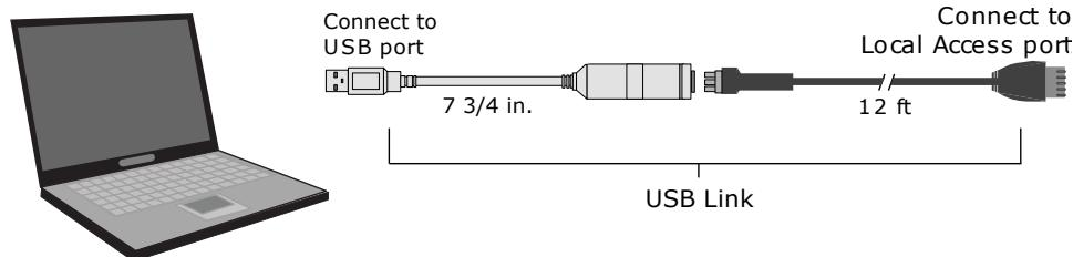
**NOTE** If using a USB isolator, plug the isolator into your computer's USB port, and then plug the USB Link cable into the isolator.
