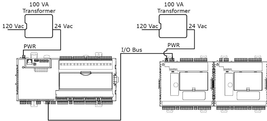
The following configuration shows a combination of connections using the I/O bus edge connector and daisy-chained wiring to the **I/O Bus** port.
