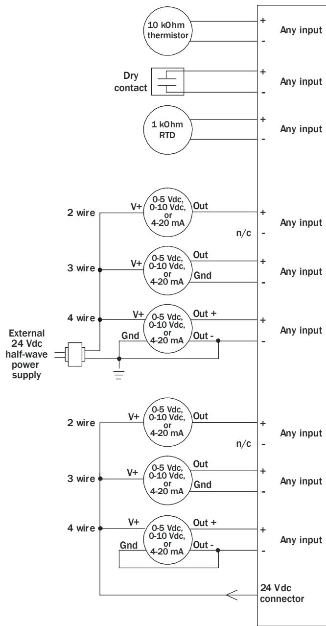
**NOTE** For a loop-powered 4-20 mA sensor, wire the sensor's positive terminal to the **+** terminal on the TV-MPCXP1628-NR's **24 Vdc** connector. Wire the sensor's negative terminal to an input's **+** terminal.
