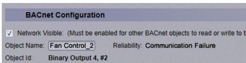
5 Anything other than **No Fault Detected** indicates an error. See the table below to determine the error and possible actions to take.
