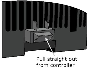
**⚠️ WARNING** This connector provides power and communication. To prevent risk of shock, do not touch the bare edge connector if the controller's power is on.
