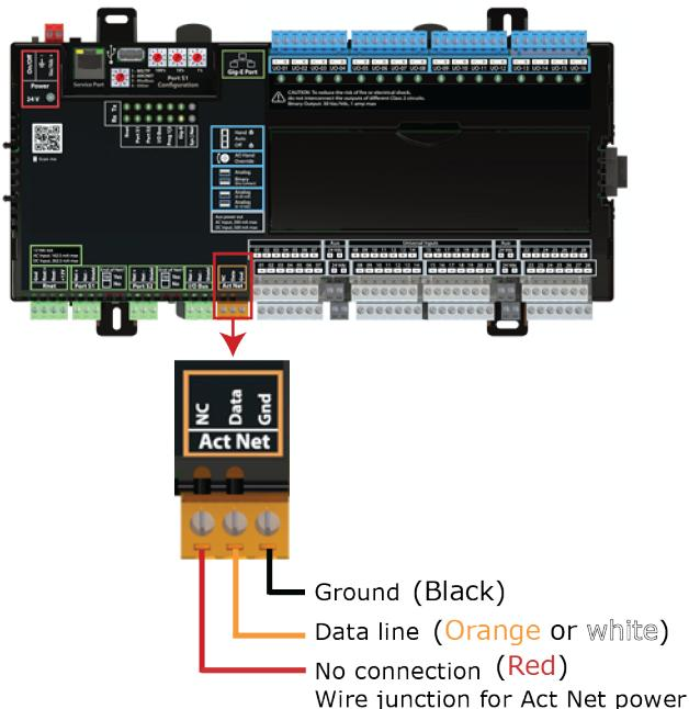
The Act Net port's **NC** (not connected) terminal does not connect to any internal circuitry. It is strictly for terminating wires in a daisy chain bus configuration.
