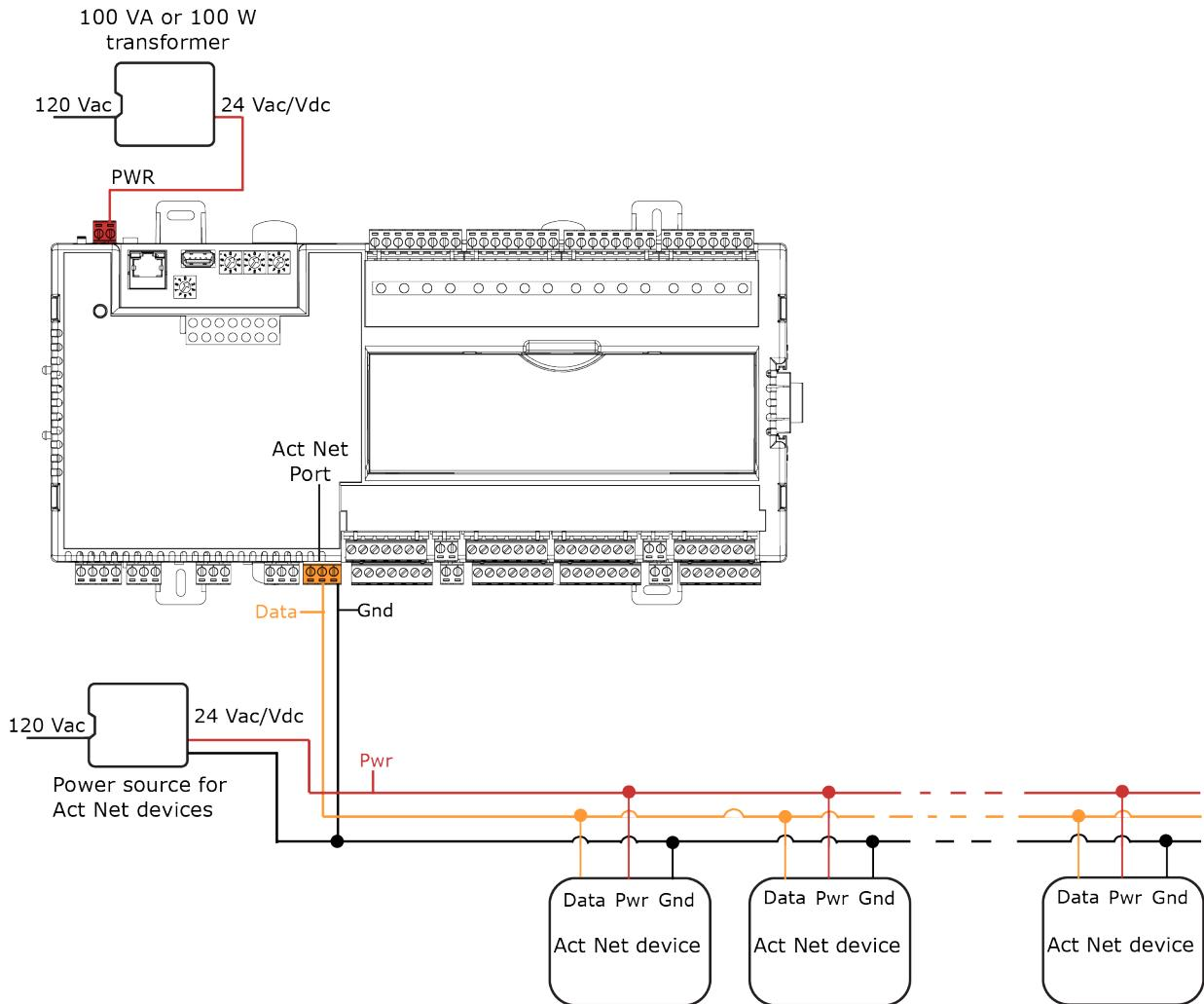
Act Net communication to the Act Net devices on a bus has a maximum length of 300 feet (91.44 meters). The bus should be wired with copper conductors of an appropriate size (18 AWG or larger) to compensate for voltage drop and ensure that bus voltage does not drop below 19.2 Vac or 21.6 Vdc.
