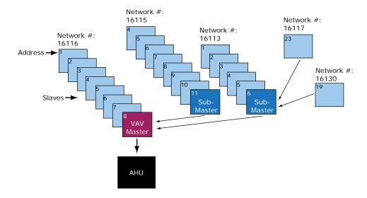
You set up linkage for the system by defining the Linkage properties for each controller. See *Linkage Properties* (page 68).
