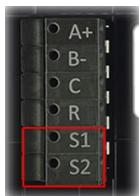
Use Remote Sensor input terminals S1 and S2 for the following inputs:
