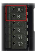
Connect communication wiring to terminals **A+** and **B-**. Do not terminate shield at the thermostat.
