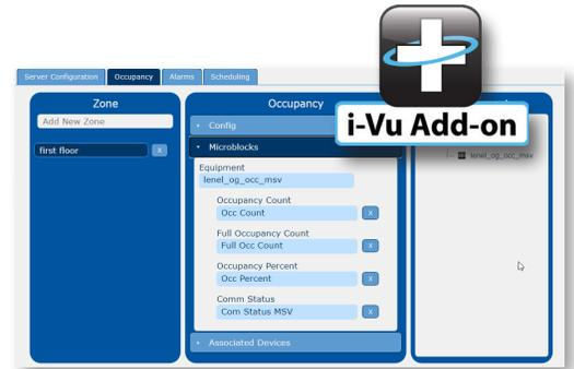
The OnGuard integration consists of a collection of add-ons that allow the i-Vu building automation system and an OnGuard security system to work together. The OnGuard integration solution consists of three add-ons that you can purchase based on your integration needs.
