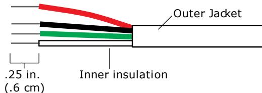
**3** Wire each terminal on the sensor to the same terminal on the controller. See diagram below.
