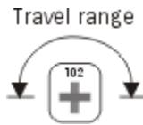
**WARNING!** The output potentiometer is NOT used for binary output channels. For a binary output, turn the potentiometer clockwise until it stops (maximum output) and leave it in this position. Failure to do so may result in relay-chattering or failure of the relay to energize when the **Auto-Off-On** switch is in the **On** position.
