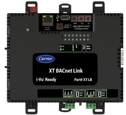
The i-Vu® XT BACnet link allows you to integrate other manufacturers' equipment into the i-Vu building automation system using BACnet and/or Modbus protocols, making it easy to tie in equipment such as VFDs, boilers, and lighting systems. Each i-Vu XT BACnet link supports up to 1,500 third party BACnet points and up to 500 Client/Server Modbus points using Modbus/IP or Modbus RTU protocols.
