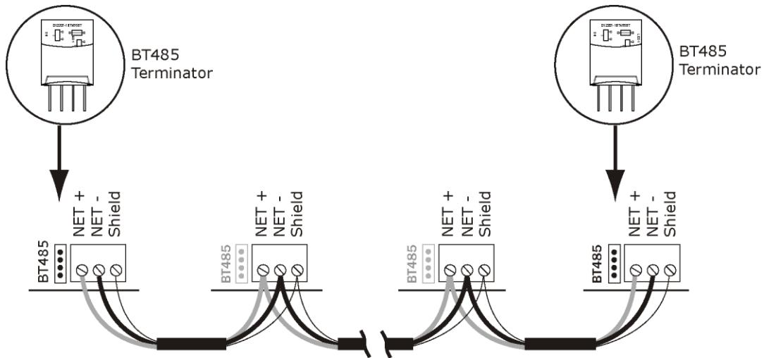
See the *MS/TP Networking and Wiring Installation Guide* for more details.
