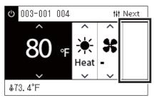
A blank is displayed if there is a function whose settings cannot be changed. The screen shown at the left is an example of the model having a fixed louver. Blank spaces cannot be selected using [<] or [>].
