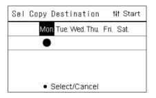
4 After selecting the copy destination, press [14] (Control). "Copy Complete" is displayed, and the "Weekly Schedule" screen is displayed again.
