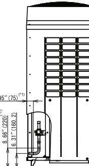
(\*1)Cutting position of L-shape pipe
