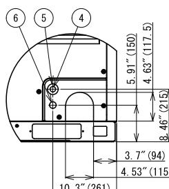
Holes for piping/wiring
