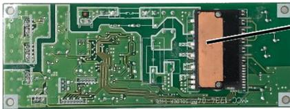
Uniformly apply the Silicone Thermal Grease to the heat dissipating surfaces of the IPM (IC300).
