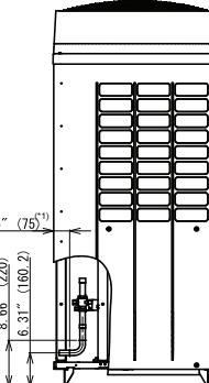
(\*1)Cutting position of L-shape pipe
