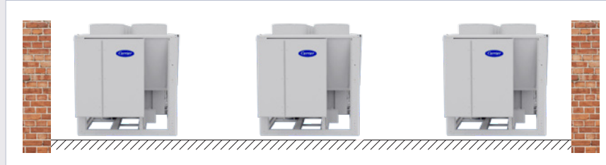
Chillers side by side with brick walls at the end
