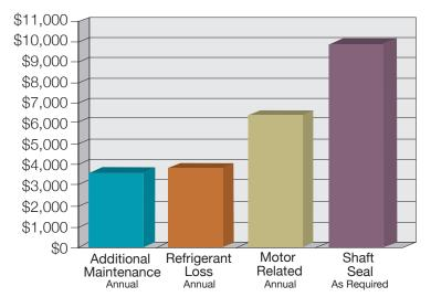
Additional Maintenance includes cleaning oil cooler, weekly inspection of shaft seal and replacing VFD glycol.
