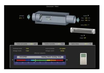
temperature and CO<sup>2</sup> sensors in each classroom and office, have enabled the existing split system to create a positive-pressure indoor environment with ventilation precisely controlled for occupancy, while reducing energy demand by one-third.
