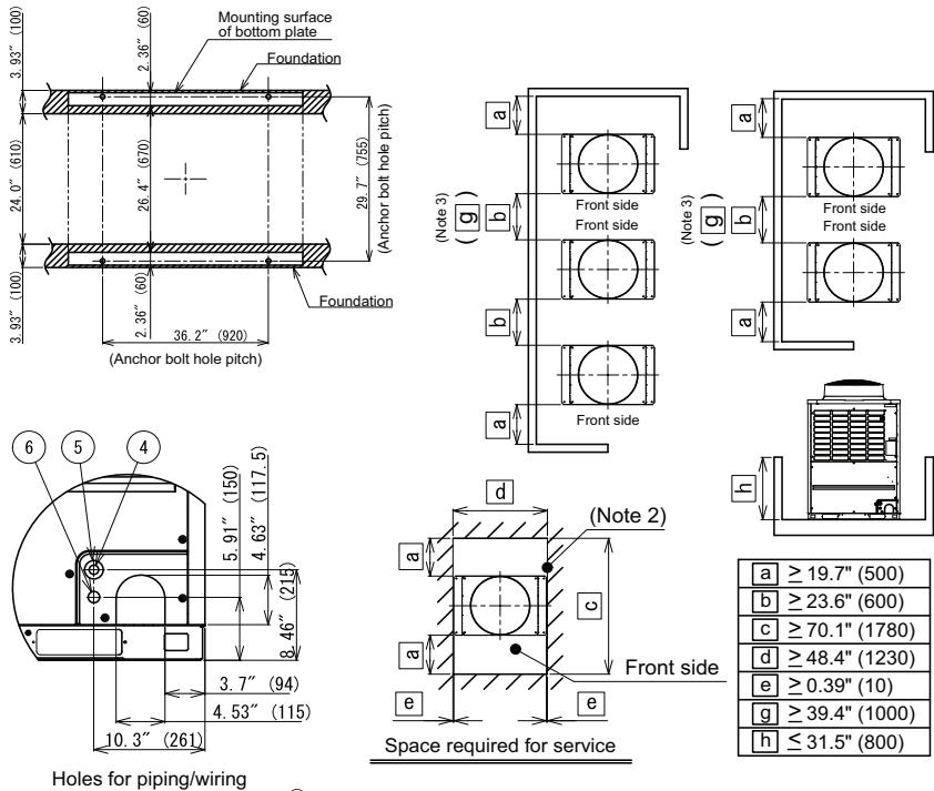
Holes for piping/wiring
