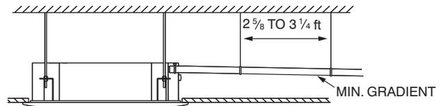
**Fig. 11 — Condensate Piping**
