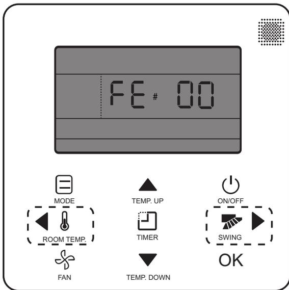
**Fig. 30 —Non-Programmable Controller IDU Addressing Menu**
