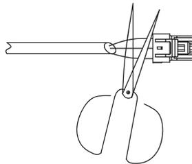
**Fig. 22 —Shearing Outdoor Connector**
