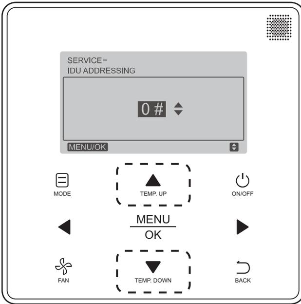
**Fig. 33 —Programmable Controller Setting IDU Address**
