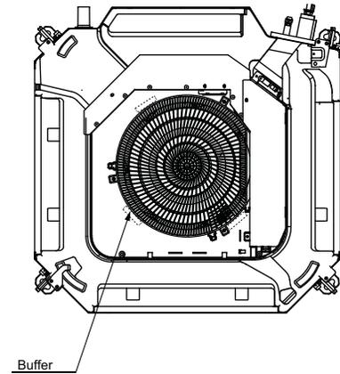
**Fig. 6 —Example of Buffer Locations**
