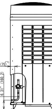
(\*1)Cutting position of L-shape pipe
