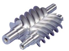
the refrigerant. As the rotors turn, the gas is progressively compressed in decreasing volume along the length of the screws. This continuous, smooth compression process reduces pulsation and mechanical stress.
