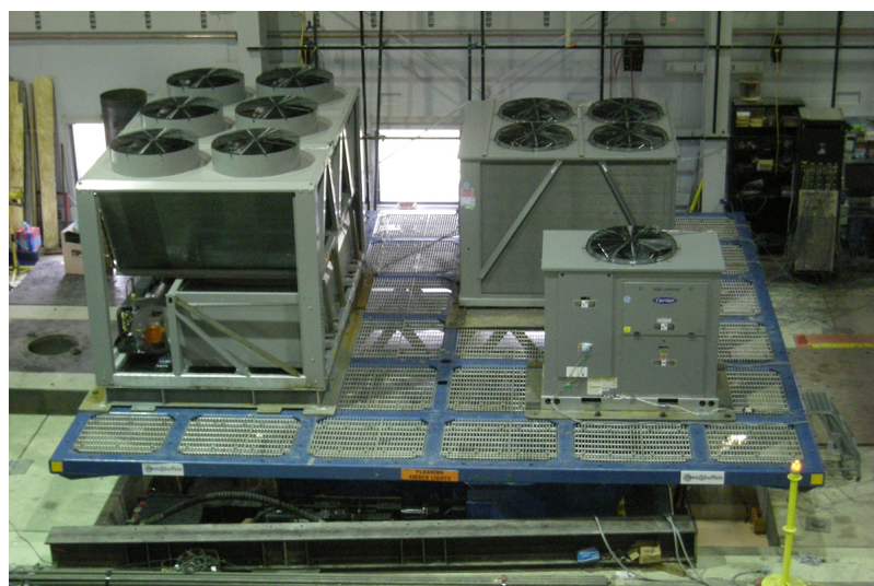
Figure 2: Carrier Products on Three Dimensional Shake Table
