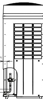
(\*1)Cutting position of L-shape pipe
