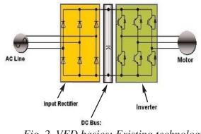
Fig. 2. VFD basics: Existing technology
