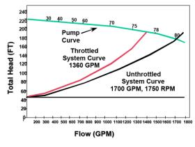
Fig. 3. Mechanical capacity control
