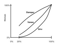
Fig. 4. Comparison of mechanical capacity control and speed capacity control
