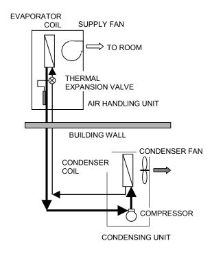
Figure 1. Typical Split System Schematic
