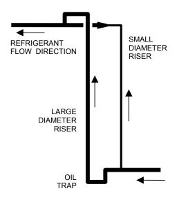
Figure 2. Typical Double Riser Arrangement
