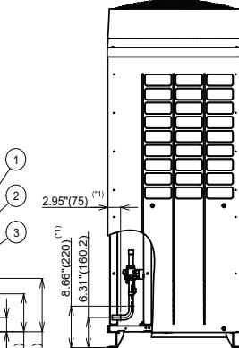
(\*1)Cutting position of L-shape pipe
