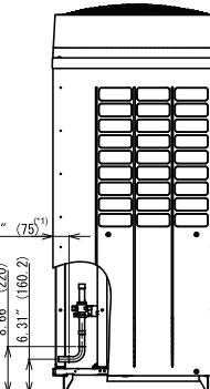
(\*1)Cutting position of L-shape pipe
