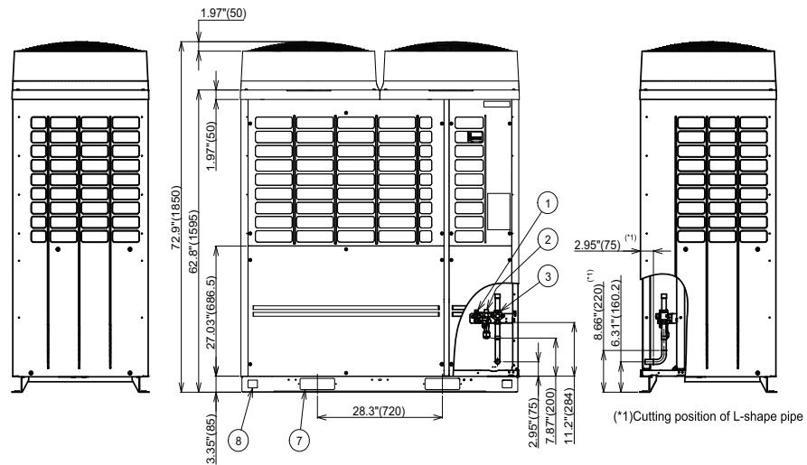
(\*1)Cutting position of L-shape pipe
