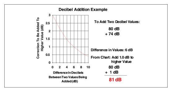
More importantly, most people cannot differentiate between two sources which differ by less than 3 dB. If the background sound is an NC-35, and the device in question is predicted at an NC-35, it is likely that the space will be at an NC-38 (although this is dependent on which octave bands are critical), but most people cannot hear the difference.
