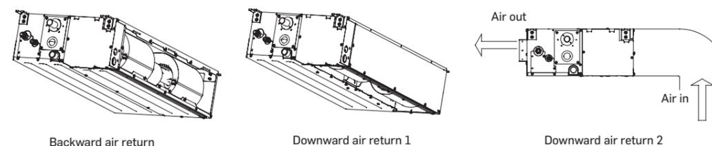
Note: the downward air return mode would increase noise 3-5 dB(A). It is recommended to install the air conditioner in downward air return mode 2 if enough space is available.
