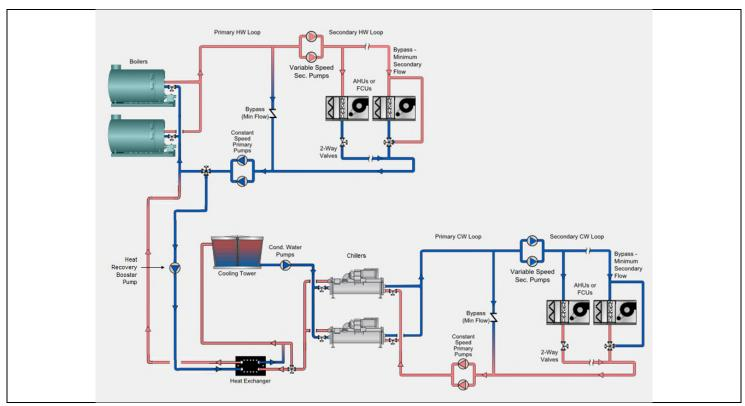
Figure 1. Diagram of Heat Recovery Plant with Heat Exchanger in Condenser Loop (Note: This is a simplified diagram only intended to show the basic arrangement of components)
